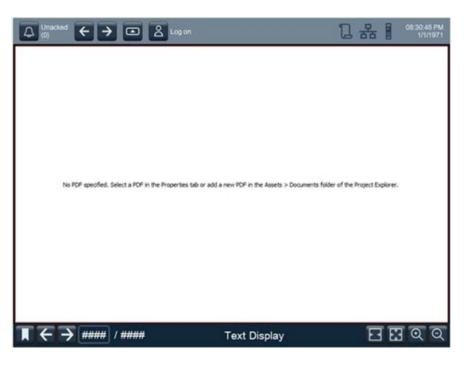
Tip: Expanding the Assets > Add-On Graphics folders and then dragging the PDF\_Viewer Add-On Graphic or rightclicking the PDF\_Viewer Add-On Graphic and selecting Add Add-on Graphic to (screen name) also adds a PDF Viewer Add-On Graphic to a screen or popup from Project Explorer.
