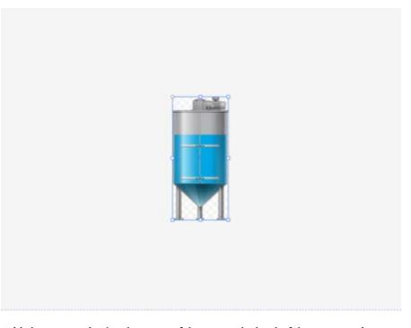
Add elements to display the name of the mixer, the level of the mixer, and a numeric input to specify the level set point. When adding elements to the add-on graphic definition, the checkerboard pattern shows the size of the graphic.
